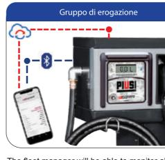
CUBE 70 B.SMART Electronic delivery group with nominal flow rate 70 lt / min, equipped with self-priming pump with built-in filter, digital flow meter with +/- 0.5% accuracy, delivery hose mt. 4, automatic dispensing noozle and minimum level pump
